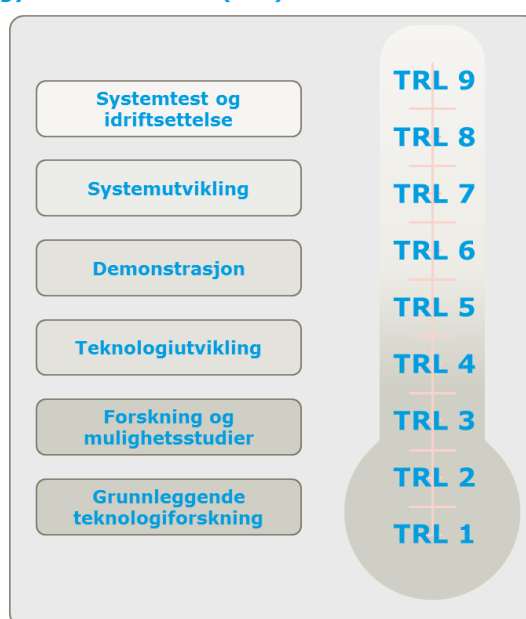
Figur 5.3 – Skala for teknologimodenhet, Technology Readiness Level (TRL)
